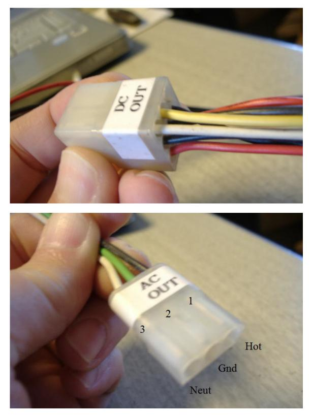
The AC output connector is intended to feed 120 volts AC to the rest of the cabinet to operate the marquee light fixture, monitor isolation transformer, and dollar bill acceptor (if equipped). This connector is controlled by the power switch.
