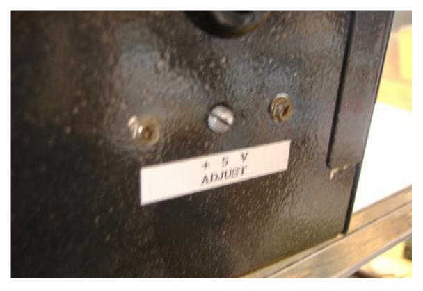
The +5 volts adjustment pot is located on the side of the case. If the shaft is too short to grab with your fingers to adjust it, use a small straight slot screwdriver instead to turn it.
