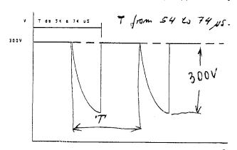
Check the same signal but now pressing the **RESTORER G** (SW9) [23] key, changing the probe ground connection to **G** (pin8-J1).
